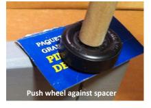
until the inner wheel hub touches the spacer; then remove the spacer. Repeat for the other wheels and they will all end up spaced evenly from the car. When doing the other side, avoid putting pressure on the wheels you just spaced by blocking up the car body so the wheels don't touch the work surface.
