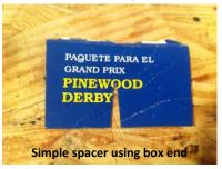
create a spacer by tearing off the flap of the PWD kit box and cutting a 1/2" long narrow V groove. Slip the axle through the wheel, insert the axle part-way into the slot and slip the spacer groove all the way onto the axle and hold it against the car body. Using that dowel from #4 above, slowly push the axle in by hand
