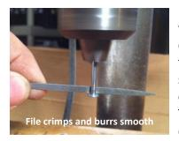
Put each axle in a drill press or secured handheld drill to smooth them out while they spin. Starting with a small fine file, remove those tiny parallel
