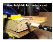
Third, **drill holes for the weights**. The easiest to install are the round, notched lead weights (but tungsten is better). Drill a test hole in a scrap of wood and check that the weight fits smoothly (usually 7/16" to 1/2" diameter). With the correct sized bit, drill the holes in the locations as explained in #2 above, keeping in mind your design and where you will be removing wood later
