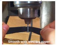
reflection in the top half of the axle! Finish off the shaft by spinning on some dry lubrication (see #9 below) with a soft cotton pad.
